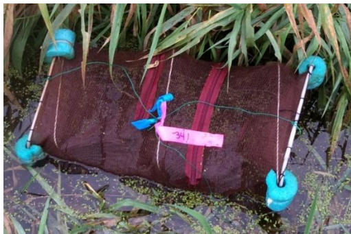
Figure 1. Left: Soft-sided minnow trap fitted with pool noodle pieces. Right: standard Gee style minnow trap.
