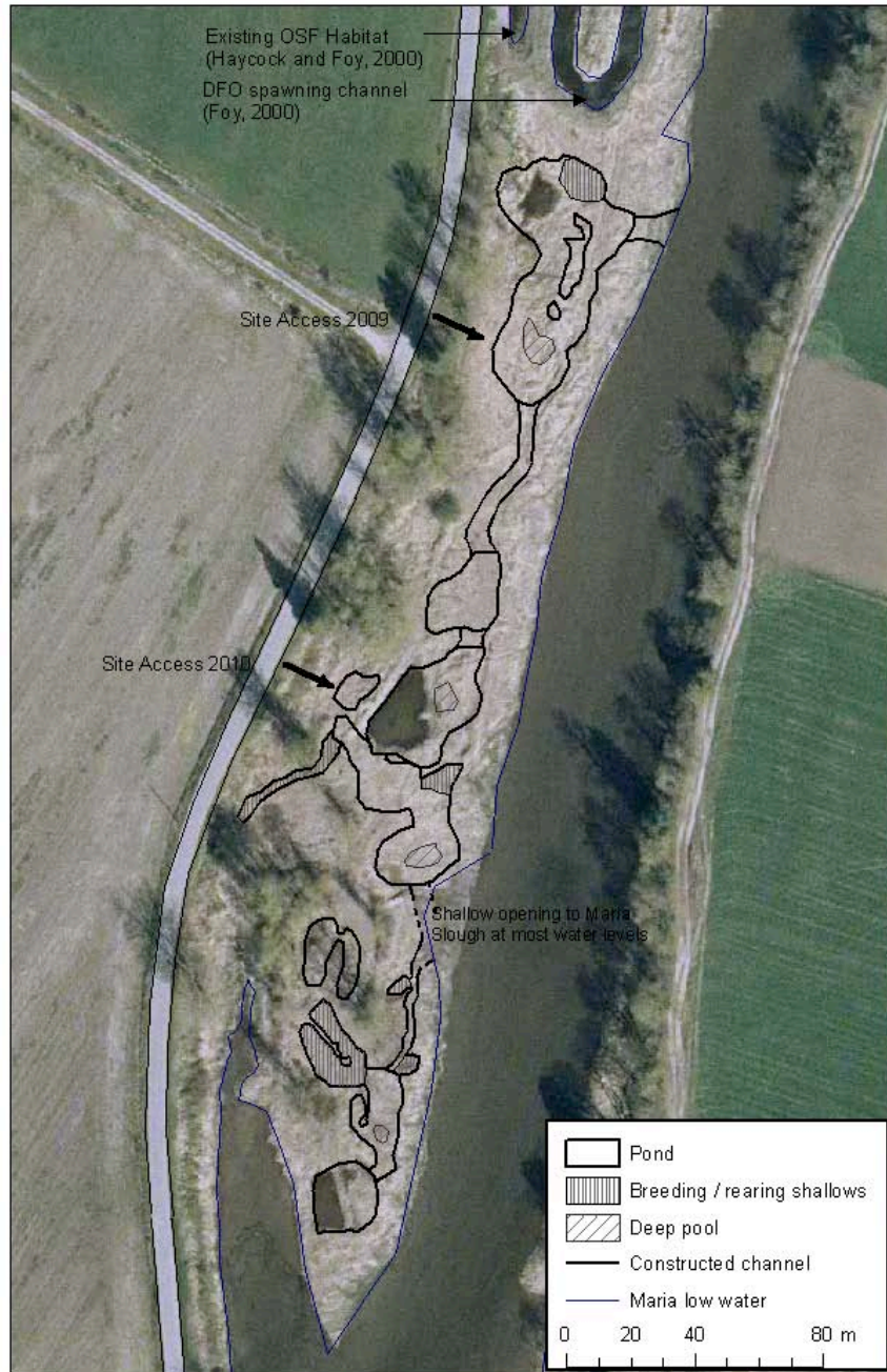
Figure 4. Overview map of wetland construction completed in October 2010.
