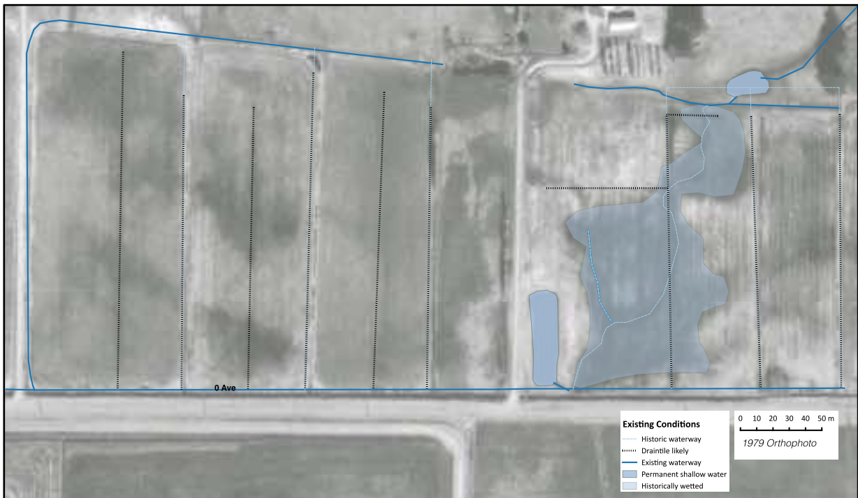
Figure 9. Existing hydrology indicating location of drain tile as identified on 1979 orthophoto.
