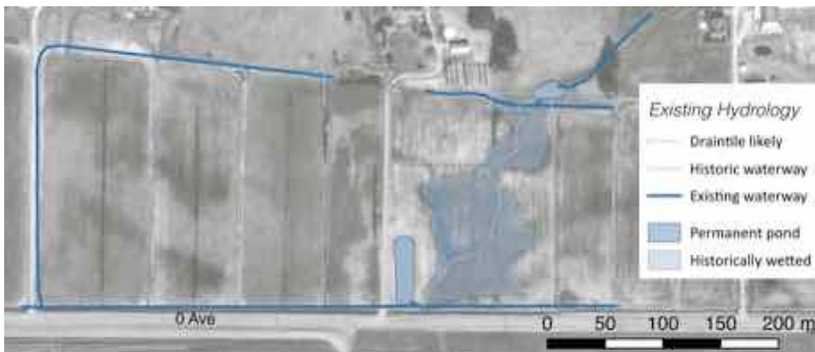
Figure 5. Location of existing and historic drainage features, overlain on orthophoto image from 1979.
