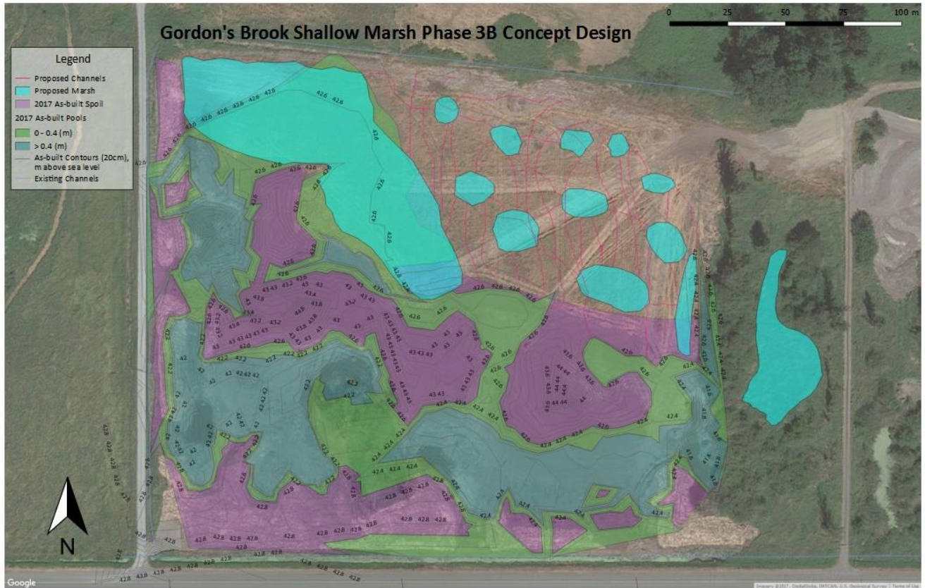
Figure 9: Concept design for Phase IIIB, complexing the north-east corner of the field and constructing additional ponds in the east sector.
